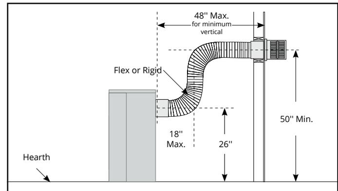
Figure 9.c Rear Vented, wall mounted Multi-elbow termination installation. Multi-elbow venting installation for H\*34DF\* must have a minimum vertical rise of 50". The vent run must comply with the Venting Graph
