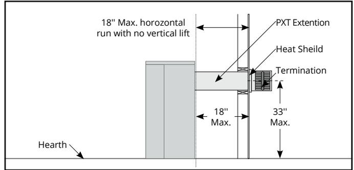
Figure 8.m Straight run, Rear Vented, wall mounted termination
