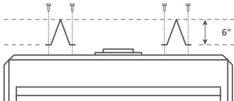
Figure 4.b Installing standoffs
