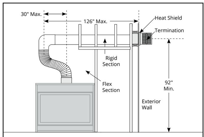
Figure 8.d Top Vented, wall mounted Retracted Multi-elbow installation
