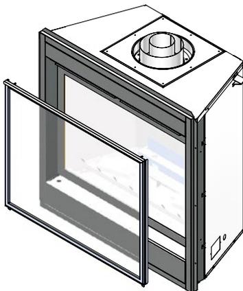
Figure 19. Lift out the Retaining Tabs and screen
