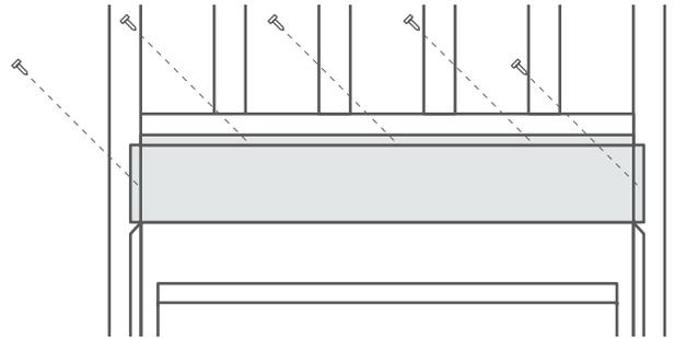
Figure 4.c Installing standoffs
