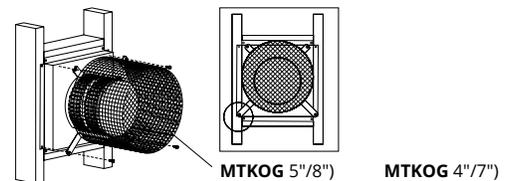
Figure 7.f Installing a MTO, PTO termination heat guard.
