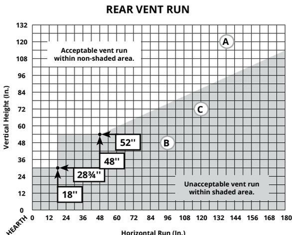
Figure 8.i Rear Venting Graph for wall mounted terminations
