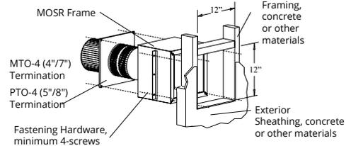
Figure 7.d Installing a PTO termination with MOSR frame.
