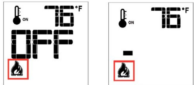
Figure 27.g Flame Off and Flame Level 1.
