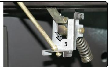
Figure 20.f Lift the latch upward
