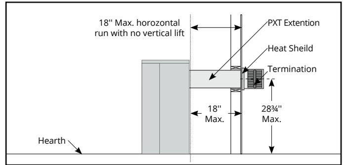
Figure 8.j Straight run, Rear Vented, wall mounted termination
