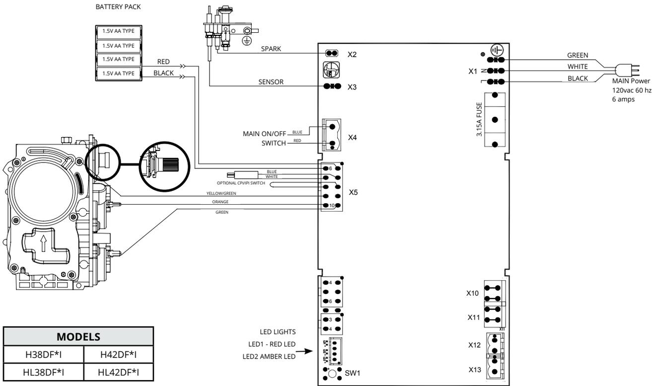
Figure 16.b Wiring diagram for SIT Proflame 2 Electronic Ignition
