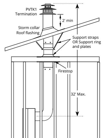
Figure 6.d Side vent, Roof mounted venting (1 = 90° bend).
