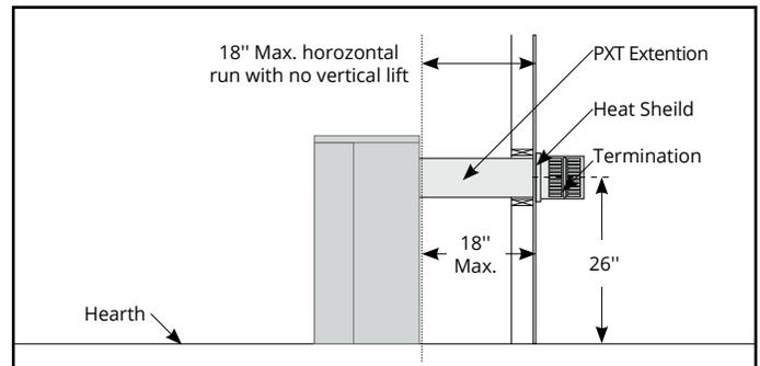
Figure 9.b Straight run, Rear Vented, wall mounted termination.
