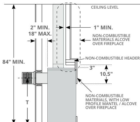
Figure 3.d Non Combustible Framing with alcove above fireplace
