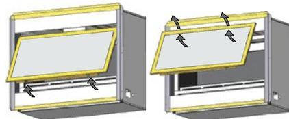
Figure 20.h Removing and installing the glass doors.
