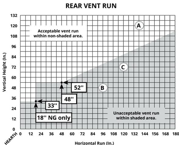
Figure 8.1 Rear Venting Graph for wall mounted terminations
