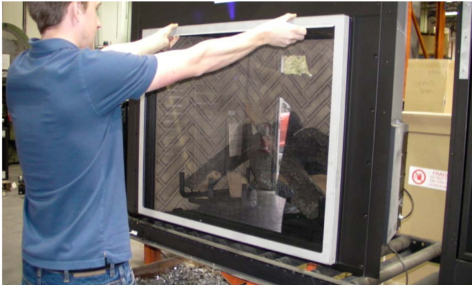
Figure 16. Lifting top edge of screen.
